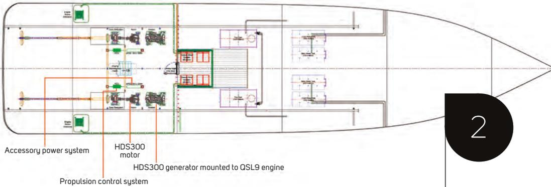
1. The AC traction motor can generate up to 6,000Nm of torque immediately for the propeller, and speed can be precisely controlled from 1rpm on the shaft up to maximum speed, providing unmatched response and control
