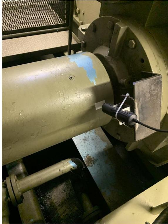
Information from each fuel meter and RPM sensor was transmitted directly into a data acquisition system and recorded at a 1 Hz frequency. The datalogger used for testing is shown in Figure 4.
